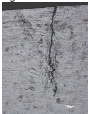
Figure 2. Branched transgranular cracking initiating from ID. Figure 3. Transgranular fracture surface.
